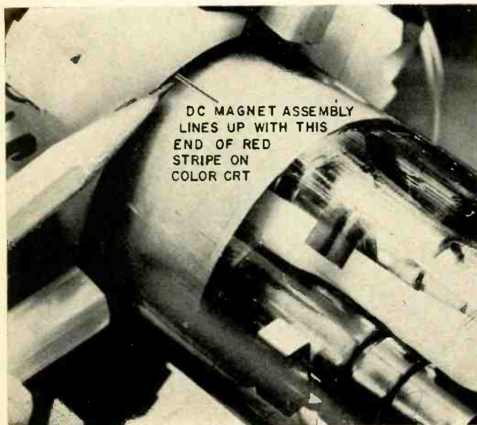
Dc magnet assembly is lined up at this end of red stripe on color CRT
