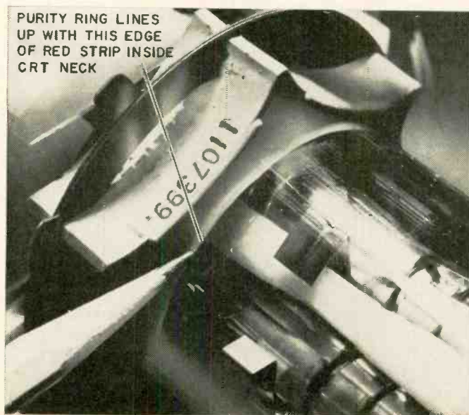
Center purity ring is lined up with red stripe on neck of CRT.
